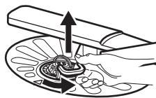
To remove filters (B) and (C), turn the handle counterclockwise and pull it upwards. Remove the filter (C) out of filter (B). Wash the filters with water.
