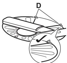
Put the flat filter (A) back in place. Make sure that it is correctly positioned under the 2 guides (D).
