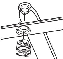
Insert the mounting element in the spray arm and fix it in the delivery tube by turning it clockwise. Make sure the mounting element locks into place.
