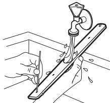
Wash the spray arm under running water. Use a thin pointed tool, e.g. a toothpick, to remove particles of soil from the holes. Run the water through the holes to wash soil particles away from the inside.
