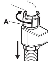
Disconnect the hose. Turn the fastener A clockwise.
